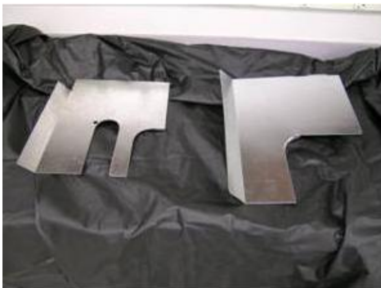
Incorrect Heat Shield - Correct Heat Shield
