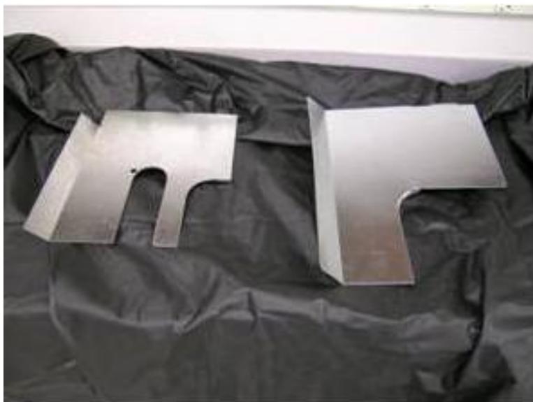
Incorrect Heat Shield - Correct Heat Shield
